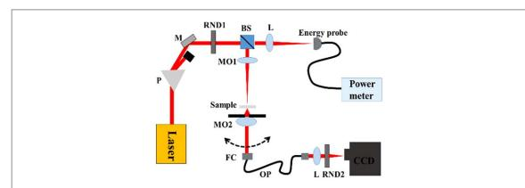
**Figure 3.** The setup of angle resolved PL. (P: prism; M: Mirror; RND: rotational neutral density filters; L: Lens; BS: Beam splitter; MO: Microscope objective; FC: Fiber collimator; OF: Optical fiber.) RND1 is the neutral density filter which regulates the excitation intensity (monitored by the power meter) and RND2 is used to prevent saturation of the detection devices. The MO<sub>2</sub> and a 400  $\mu$ m core UV optical fiber mounted on a rotating arm.
