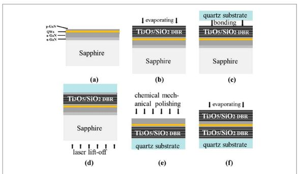
**Figure 1.** The schematic process of MC fabrication with dielectric DBRs: (a) the epitaxial wafer structure: (b) evaporating the bottom DBR on the wafer; (c) bonding to a quartz substrate; (d) removing of sapphire substrate by laser lift off; (e) polishing and thinning cavity; (f) MC structure after evaporating the top DBR.
