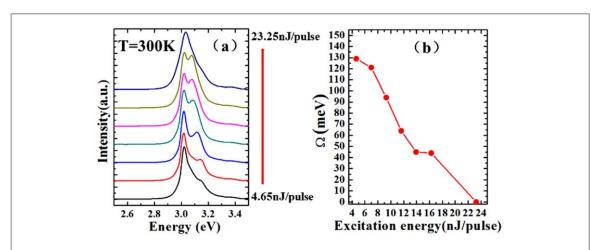
**Figure 5.** (a) PL spectra of polaritons with the excitation energy from 4.65 nJ/pulse to 23.25 nJ/pulse at room temperature. With increasing excitation energy, the UPB and LPB peaks close to each other, leading to a decrease of Rabi splitting value. (b) The Rabi splitting value as a function of excitation energy.
