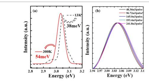
**Figure 2.** (a) Low temperature and room temperature PL spectra of InGaN QWs. (b) The normalized PL spectra as a function of excitation energy from 48.36 nJ/pulse to 241.8 nJ/Pulse.
