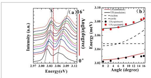
**Figure 4.** (a) Angle-resolved PL spectra of InGaN QWs dielectric MC with the angle degrees changing from  $0^{\circ}$  to  $16^{\circ}$  at 300 K. (b) Polariton energy dispersion curves as function of angle. The solid curves in (b) indicate the theoretical calculations based on a coupled harmonic oscillator model.
