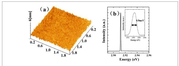
Figure 7. (a) AFM image of GaN surface after CMP with RMS roughness of 0.1 nm. (b) The PL spectrum of the cavity. The inset shows the linewidth of the emission peak.
