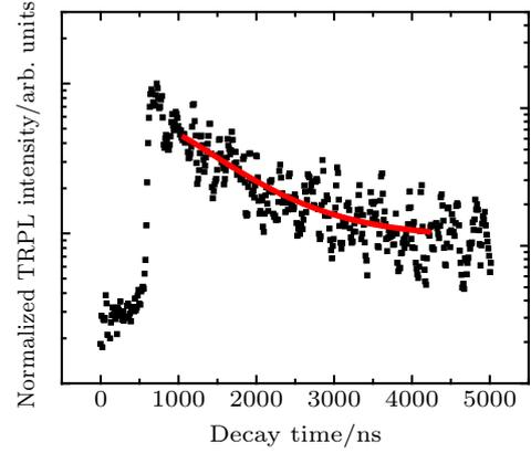
Fig. 7. Normalized TRPL intensity varying with decay time and fitted curve for green MQWs at 300 K.
