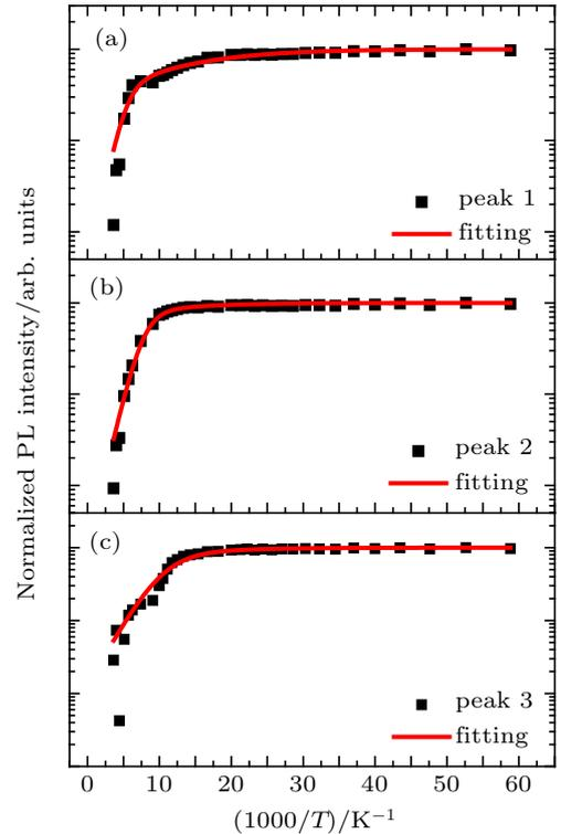
**Fig. 5.** Arrhenius plots of normalized PL intensity versus temperature of (a) peak 1, (b) peak 2, and (c) peak 3, respectively.
