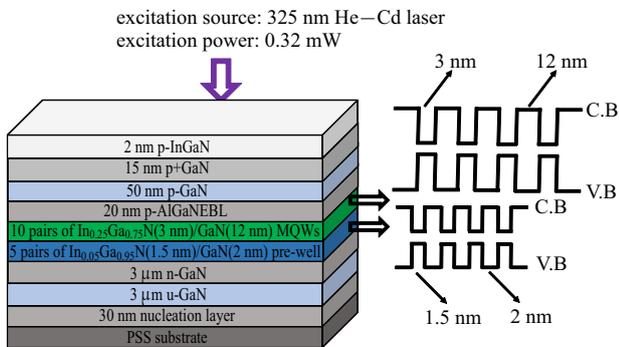
Fig. 1. Schematic diagram of green InGaN/GaN MQWs with low indium content InGaN/GaN pre-wells.
