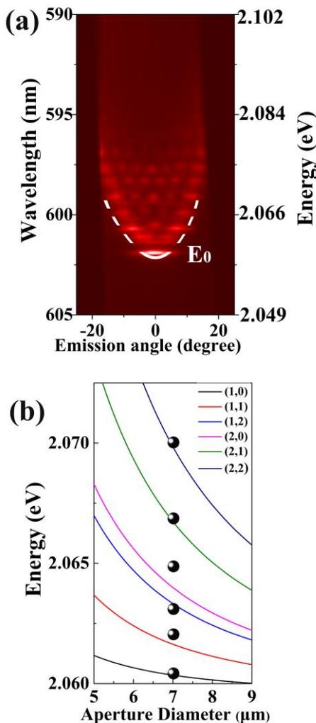
Fig. 6. (a) Emission spectrum of a single device with a 7  $\mu\text{m}$  AlN aperture diameter and a current injection of 0.03 mA at room temperature. (b) Energies
