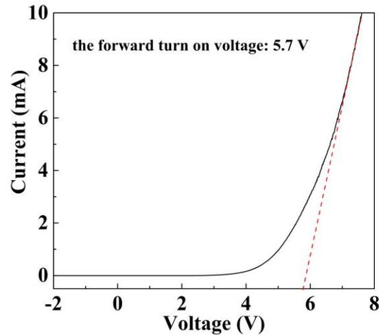
Fig. 7. The I-V curve of the orange-red RCLEDs
