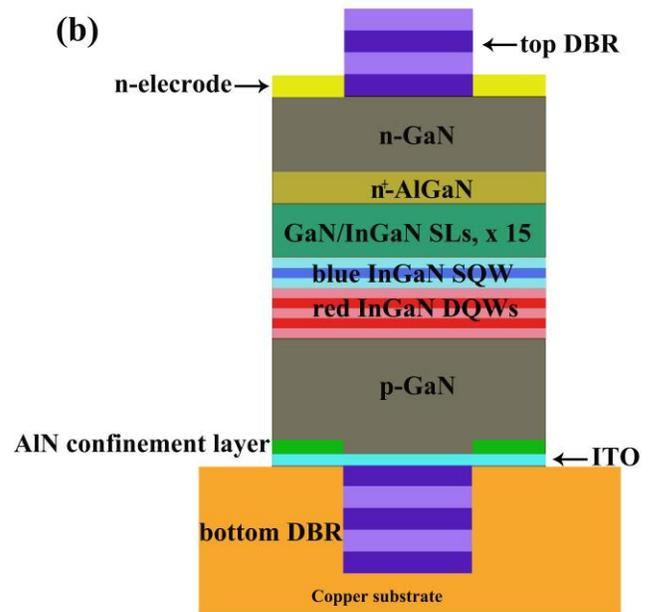
Fig. 1. (a) Schematic structure of the epitaxial wafer. (b) Cross-sectional schematic of InGaN-based orange-red RCLEDs.
