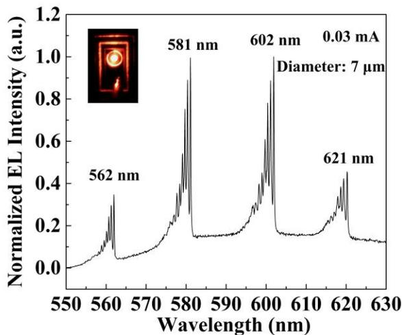
Fig. 4. Normalized EL spectrum of orange-red RCLED, with a current injection of 0.03 mA (current density 77.9 A/cm<sup>2</sup>) at room temperature. Inset is a photograph of the red RCLED acquired during EL measurement.
