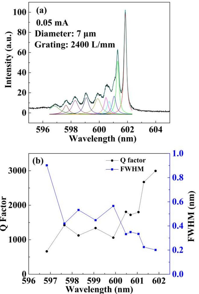
Fig. 5. (a) High-resolution EL spectrum of orange-red RCLED, with a current injection of 0.05 mA (current density 129.9 A/cm<sup>2</sup>) at room temperature and curves fitted by Lorentzian profiles. (b) Q values and FWHMs of different modes in (a).
