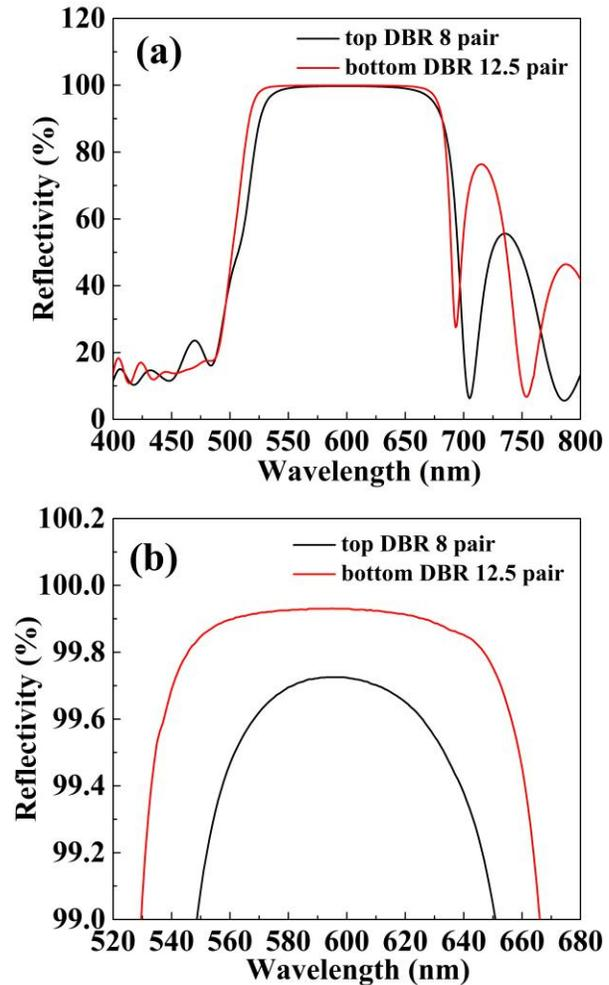
Fig. 3. (a) Reflection spectra of the top and bottom DBRs of the red RCLED from 400-800 nm. (b) Stopband of the top and bottom DBRs.
