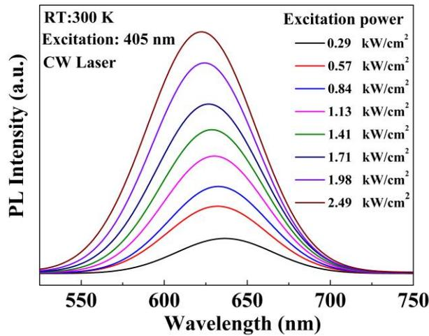
Fig. 2. PL spectra of the epitaxial wafer with varying excitation power at room temperature.
