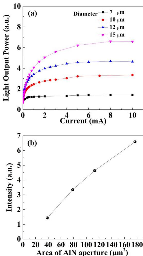
Fig. 8. (a) EL peak intensity at different currents with different aperture diameters. (b) Saturation intensity (at 10 mA) as a function of aperture area.
