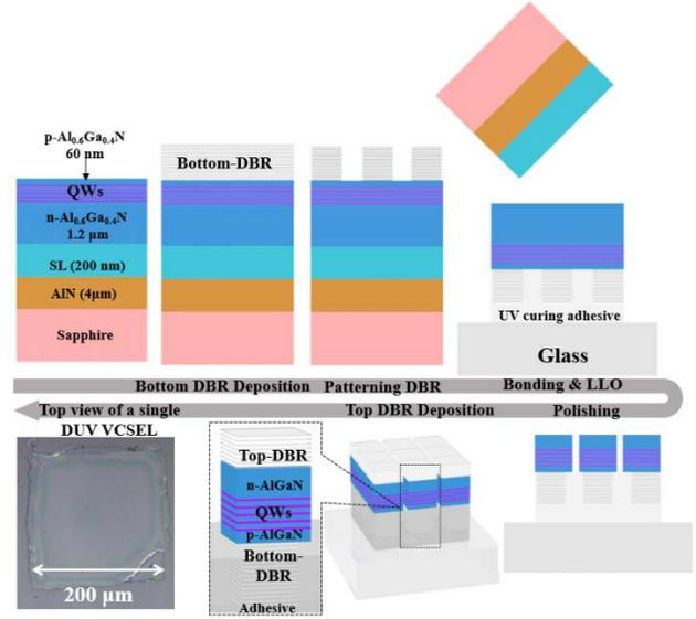
Fig. 1. DUV VCSEL fabrication process and device top view.
