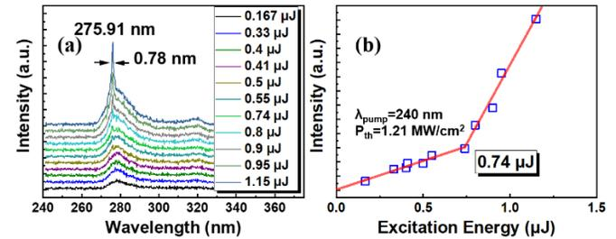
Fig. 4. Laser emission spectra for the AlGa<sub>N</sub> VCSEL with increasing pumping energy at room temperature (a), light output intensity as a function of excitation energy at room temperature (b).
