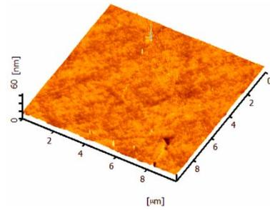
Fig. 3. AFM image (10 × 10 μm<sup>2</sup>) of the epilayer after polishing. The RMS roughness is 0.96 nm.
